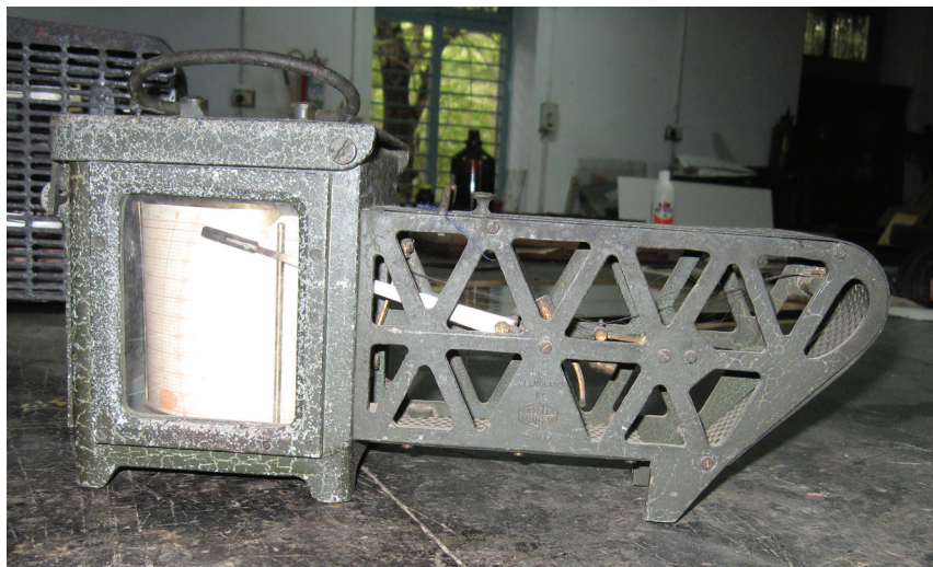
Fig. 3 The Casella hair hygograph, ca. 1937. Image by author. Published with permission from the Government Museum, Chennai.
