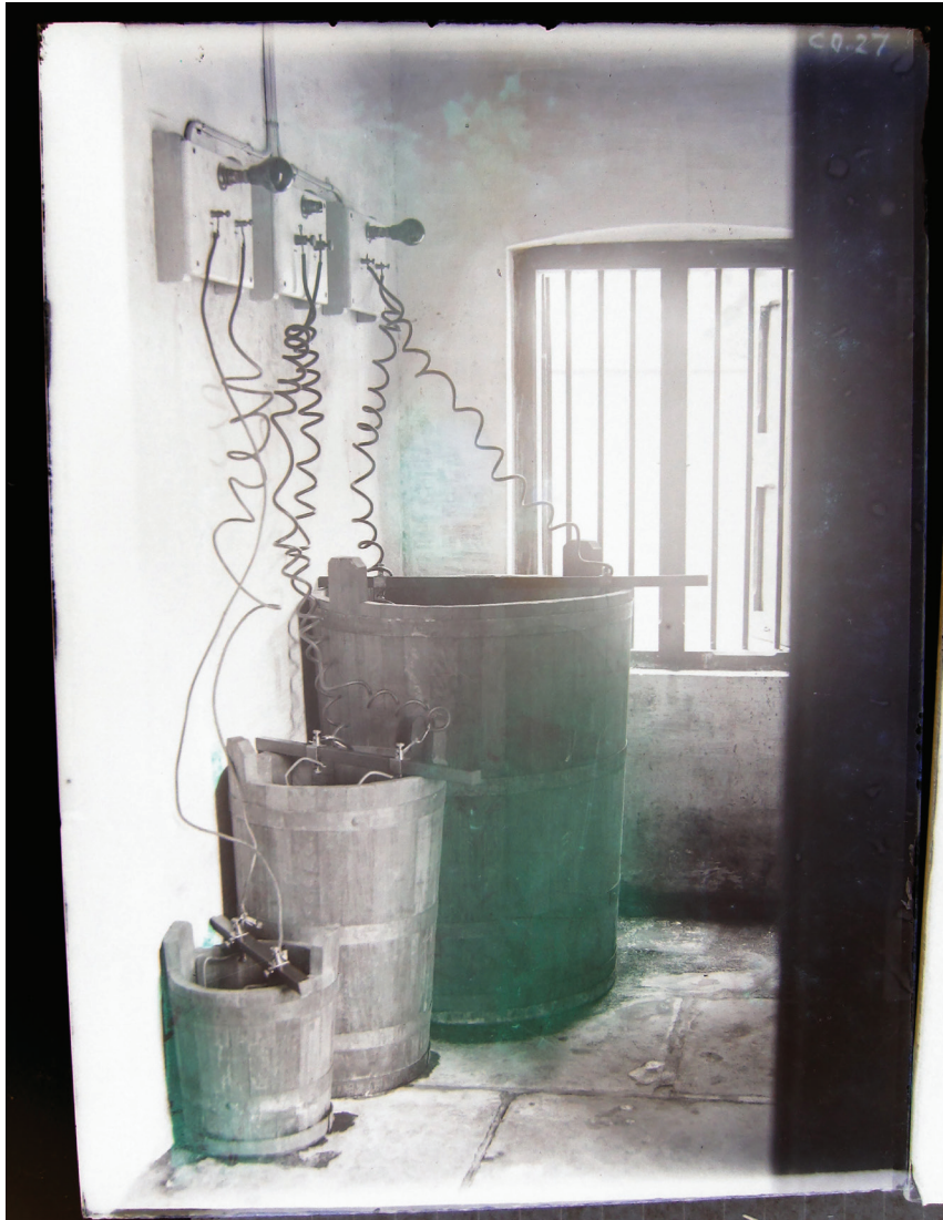
Fig. 4 View of the wooden barrels first used as electrolytic reduction tanks, n.d. Image courtesy of the Government Museum, Chennai.
